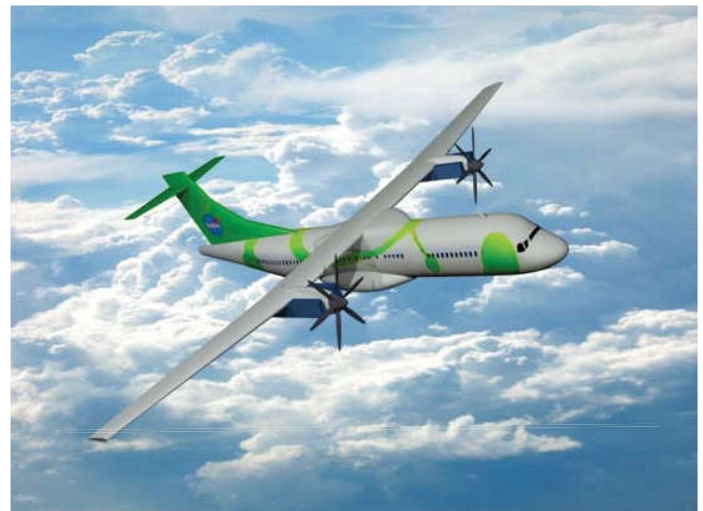
Figure 4. Rendering of the hybrid-electric ATR 42-600 in Autodesk 3ds Max. The dark blue boxes represent the location of the battery packs attached to the exterior of the nacelles.
