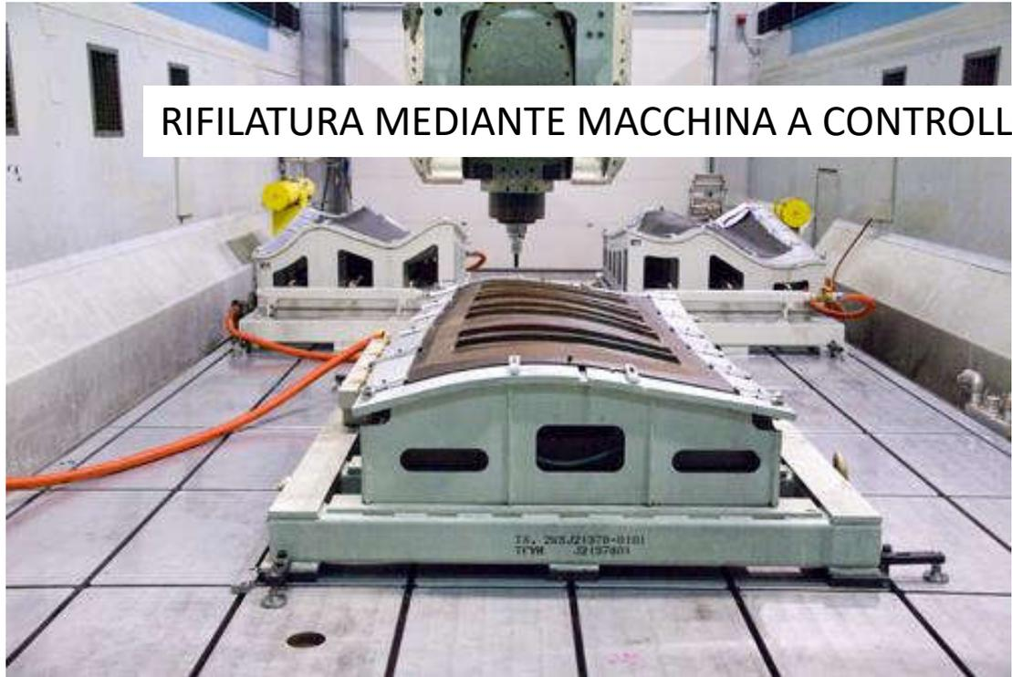
RIFILATURA MEDIANTE MACCHINA A CONTROLLO
