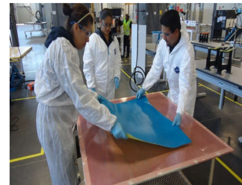
Figure 1.9 Stacking sequence of a (0/90/±45) quasi-isotropic layup.
