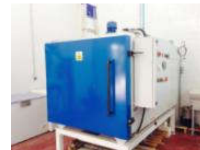
Composite Curing Oven 400° +/-2° C uniformity temperature, size [m] 1.0 x 1.0 x 1.2 with Vacuum Line.
