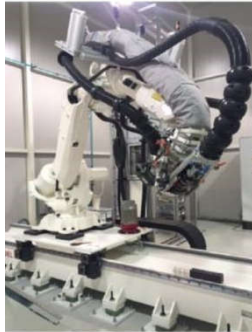
AFP Machine ABB IRB-6640/205/2.75 standard robot 8-fibre placement head, developed by Coriolis Composites s.a.s. (France), mounted on a linear axis with a working length of 3m. Material heating can be performed by a 3kW laser or IR lamp.
