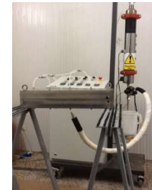
Infuser Servo injector for HP-RTM/VARTM molds, up to 4000cc per shot
